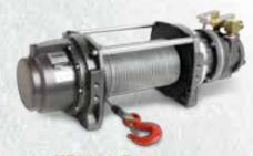
**HF3150-P** Rated to lift 3150 lbs at 21 fpm. Includes -02 drum (10" long) Wire rope supplied separately.
