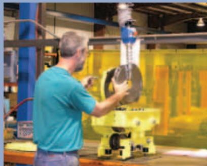
Easy Arm's optional Float Mode function allows operators to perform tasks with their hands on the load itself for maximum control.
